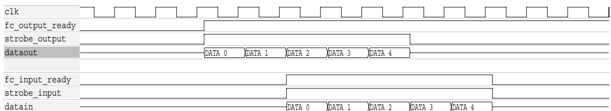
Figure 3: Signal waveform example for a simple chain of modules using the same clock
